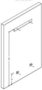
3. Place the cabinet to wall as balanced. Install the iron hanger to the wall and cabinet to make the
