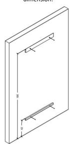
3. Place the cabinet to wall as balanced. Install the iron hanger to the wall and cabinet to make the cabinet fix.
